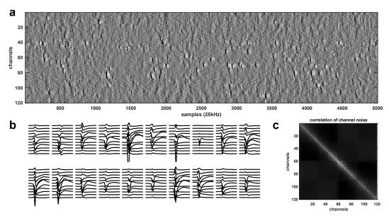
Figure 1: **Data from high-channel count recordings. a,** High-pass filtered and channel-whitened data. Negative peaks are action potentials. **b,** Example mean waveforms, centered on their peaks. **c,** Example cross-correlation matrix across channels (before whitening).
